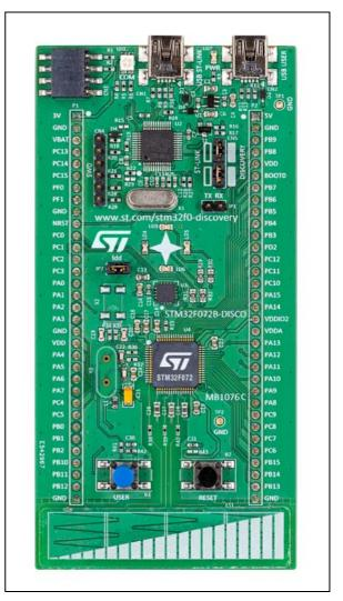
Based on the STM32F072RBT6, it includes an ST-LINK/V2 embedded debug tool interface, an ST MEMS gyroscope, LEDs, push-buttons, Linear touch sensor, touchkeys, RF EEPROM connector and a USB mini-B connector.
